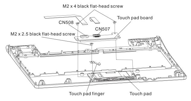
Figure 4-22 Removing the touch pad board
